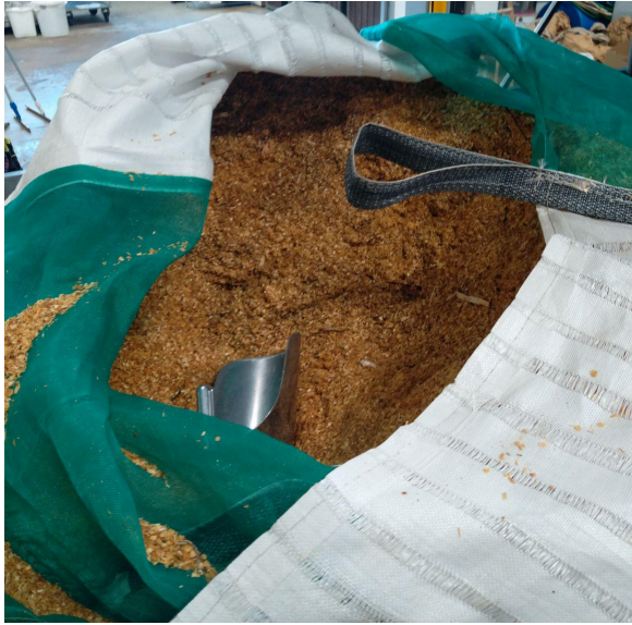
Pictures 27, 28: A big bag of birch sawdust emptied into an indoor silo for drying
