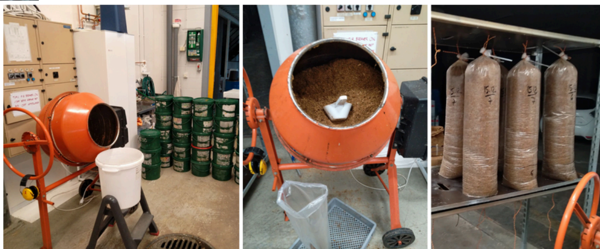
Pictures 3, 4, 5: Preparation and mixing of Hemp-based substrates
