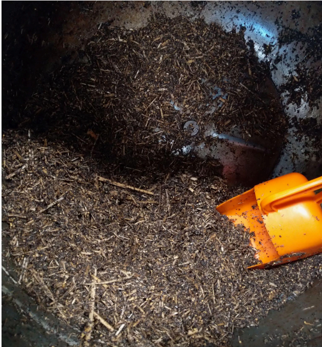
Pictures 9, 10: Long particles in substrate mixing make bag filling more difficult.
